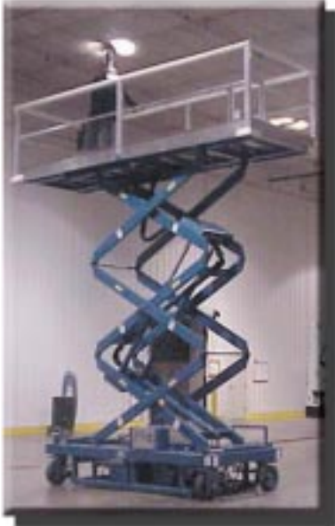
Model LPSD-2160 with custom operator platform shown in lateral drive mode.
