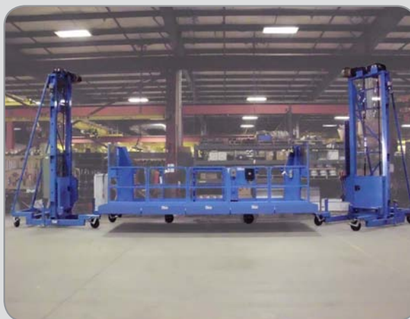
Platform with dual masts detached
