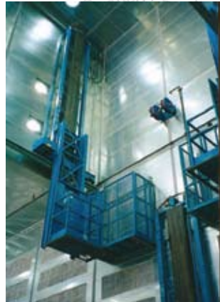
Aircraft Paint Hangar: Custom 3-Axis Lift System to access tail section of aircraft
