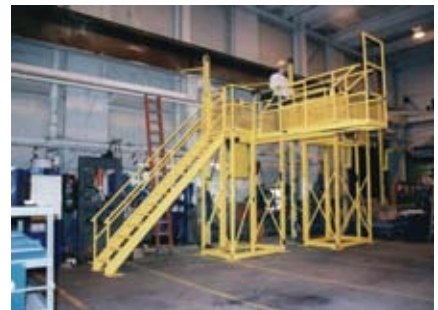
Rail Maintenance: Tip-Down Platform for locomotive maintenance
