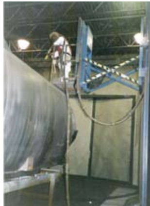
Sand Blast Booth: 3-Axis Lift Designed for blast booths using sand or steel grit
