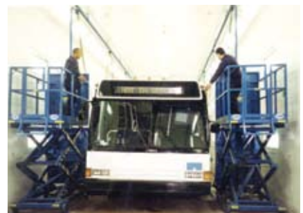
Paint/Preparation Booth: Rail Guided Scissor Lifts for paint and prep of transit buses
