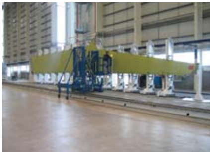
Aircraft Wing Inspection: Custom 3-Axis Lift System for aircraft manufacturer
