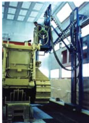
Paint/Preparation Booth: 3-Axis Lift System for painting large construction equipment
