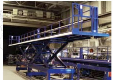
Fall Protection: Adjustable Scissor Lift Platform with safety harness used for access and fall protection while loading flatbed trailers
