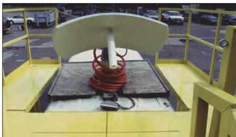
Easy access to an expanded work surface with fall protection railings improve worker safety and accessibility to roof top equipment to perform required maintenance.
