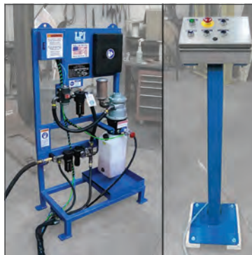
Remote Power Unit and Pedestal Controls
